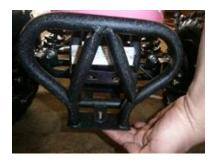
Mudguards – Place the mudguards on the bracket, then secure with the nut and bolts supplied.
