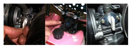
2. Pull the pull-start-handle three or four times, this will prime the engine ready to start. Pull the pull-start out slightly ensuring it is coming out straight and not at an angle, before starting the engine. Once the pull-start is in this position with a firm grip on the handlebar, the pull-start can be gently pulled to turn the engine. Ensuring not to force the pull-start out too far, as improper usage of the pull-start will damage the unit, and is not covered by the warranty.
