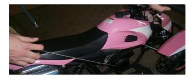
3. Once the engine has started, and runs for a few minutes, lower the silver lever (choke) to the lower position.
